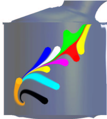
Figure 9: Dye injection is used to highlight areas of the flow in combination on the boundary surface of an intake port and combustion chamber.
